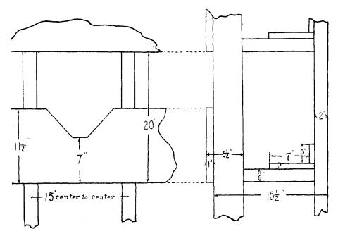
In this way a large number of bottles can be compactly stored and the solutions are easy of access. The framework structure allows the bottles to be cleaned without removing them from the rack, as they are exposed on all sides. All dirt can be brushed down into the inclined lead-lined drip trough at the base of the rack and flushed off. J. LORENZ SPORER.
